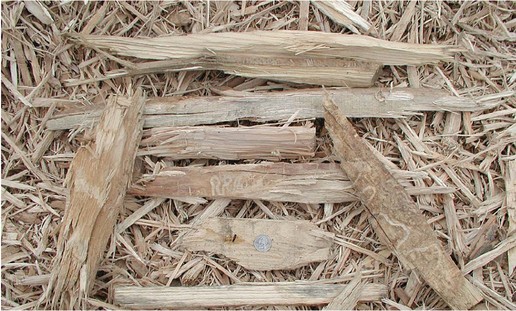
Figure 7.1 Some wood chips do not meet 2.5 cm specifications. In some larger parts, larval galleries are visible (Roberts and Kuchera, 2006).
