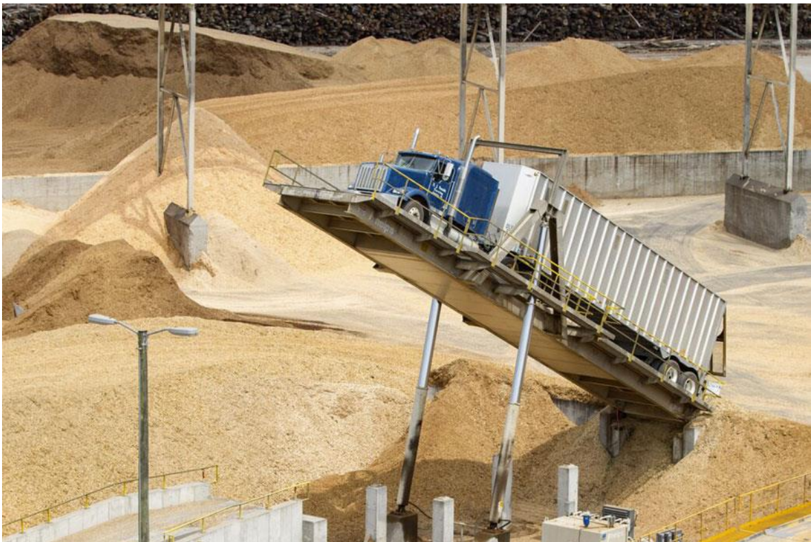
Trucks deliver logs and wood chips to Enviva's mill in Southampton County, Va., where they are heated, crushed and turned into wood pellets to be exported to Europe. Photos by Ted Blanco.
