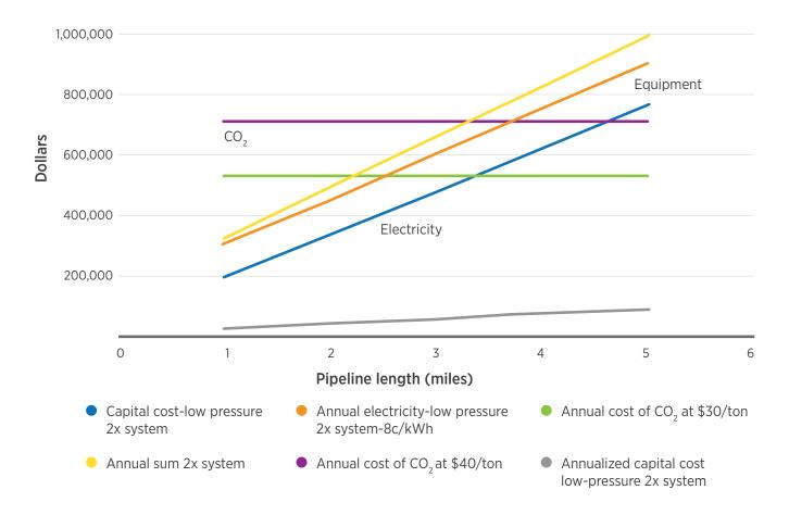
**Figure D-4** | Equipment and electricity costs for coal flue gas transport system, including two parallel sets of pipelines and blowers. The system supports a 1,000-acre open pond and is designed to minimize cost.
