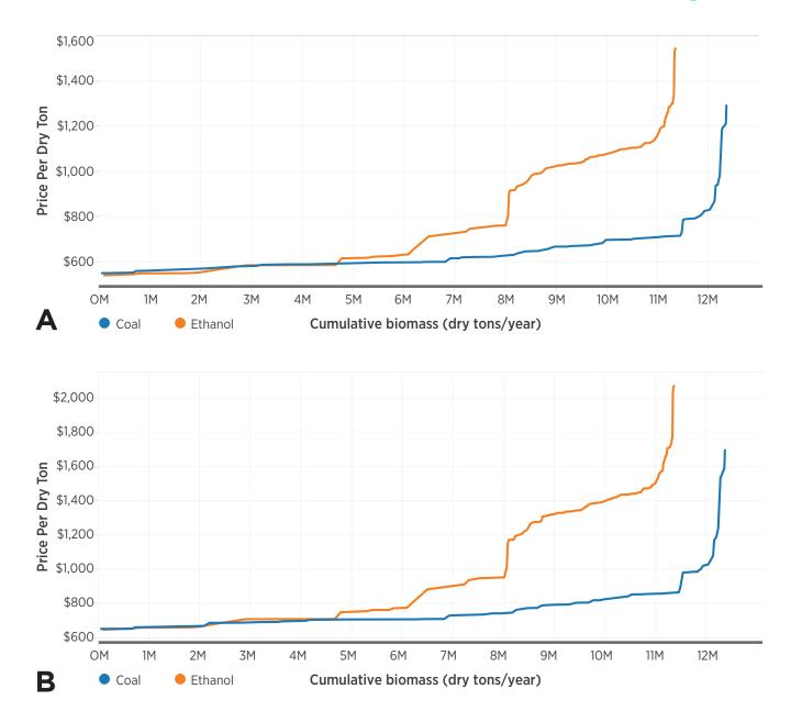
**Figure 7.35** | Minimum selling price per dry ton vs. cumulative total biomass for each co-location strategy using *Nannochloropsis salina* at future productivities for *(A)* minimally lined ponds and *(B)* fully lines ponds.<sup>11</sup>
