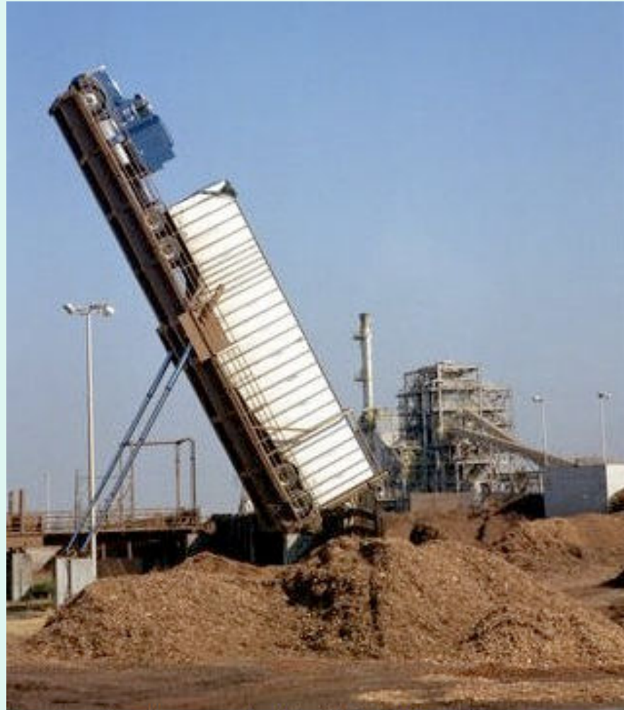
Truck unloading wood chips that will fuel the Tracy Biomass Plant, Tracy, California.
