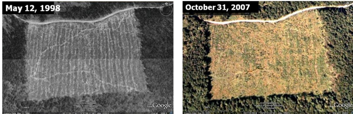
Figure 4. Repeat satellite imagery of a 25-acre clearcut in Maine, showing little regrowth after almost ten years. Assuming standard values for forest biomass in Maine, 10 the amount of wood generated by this harvest would be about 950 tons, sufficient to fuel a 50-MW biomass power plant for about 21 hours.
